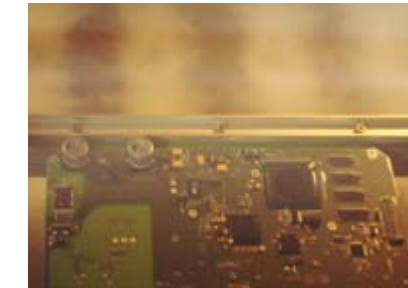
Vapour phase soldering for leaded and unleaded assembly of circuit boards
