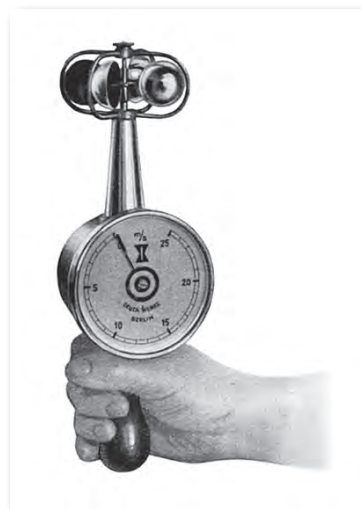
DEUTA Wind velocity indicator
